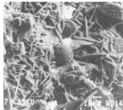
Fig. 3. Network of bladed gypsum crystals on marble traps particles to form the blackened alteration crust on marble; scale is 10 micrometers.
